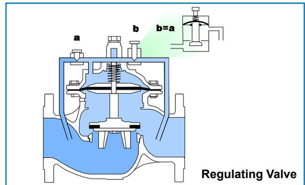
The 2-way control device provides sensitive, accurate, and constant modulating, control of the main valve. The main valve does not fully open, as the control device prevents total draining of the control chamber. The 2-way control device is standard in most pressure regulating valves.
