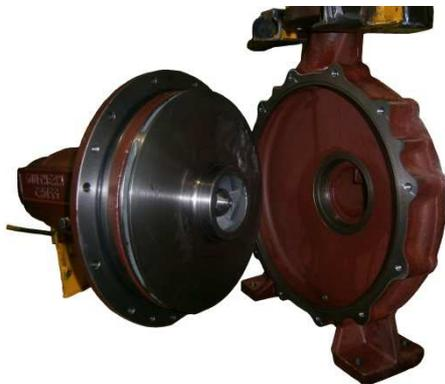
2. Unscrew the impeller nut about two turns and drive a pair of wooden or metal wedges gently between the impeller and backplate, being careful not to distort the impeller. Give the impeller nut a sharp blow, using a hammer and piece of hardwood, to spring the impeller from the taper. Remove the impeller nut and sealing washer and lift off impeller. Lift out impeller key and slide the moving section of the mechanical seal from the shaft.
